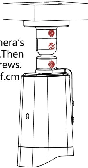
Figure 3-6 Adjusting the camera's viewing angle
