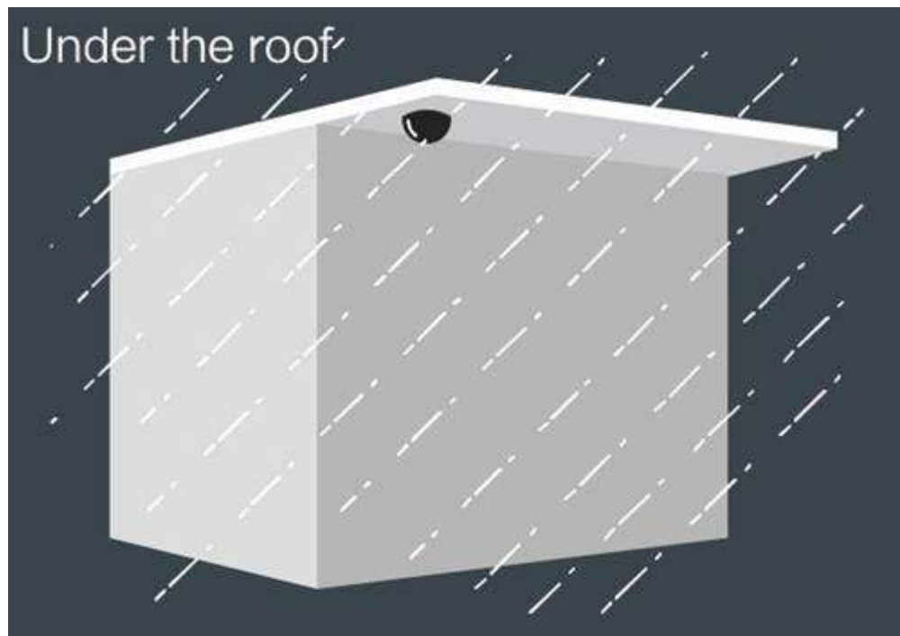
Figure 3-15 Fixed dome camera installed outdoors
