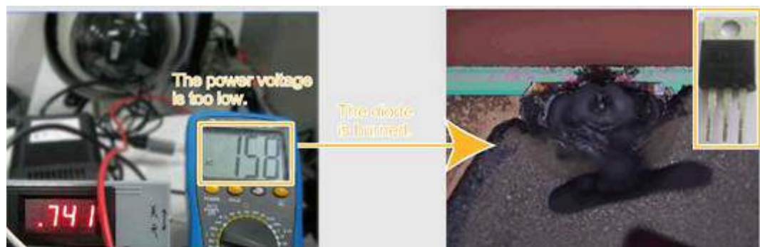
Figure 3-5 The power supply voltage is too low.
