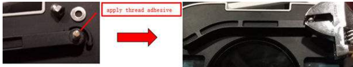
Figure 3-51 Installing the rain wiper bracket
