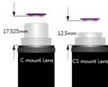
Figure 4-162 C mount and CS mount
