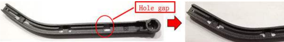
Figure 3-50 Replacing the rain wiper rubber strip
