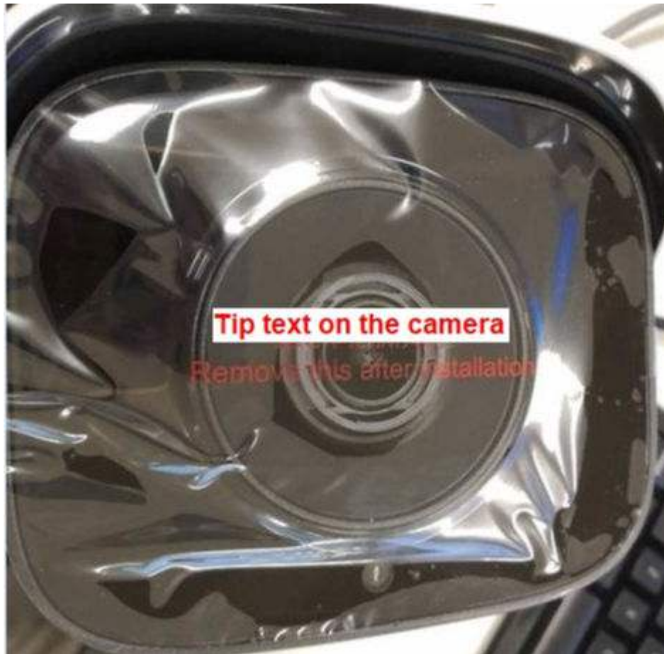
Figure 3-40 Removing the protective film after the installation
