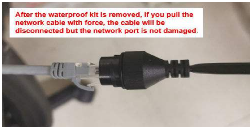
Figure 3-34 Network port is not damaged after the waterproof kit is removed
