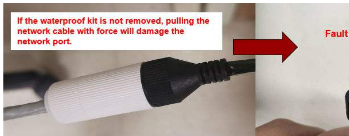
Figure 3-33 Network port is damaged after pulling the network cable forcibly without removing the waterproof kit
