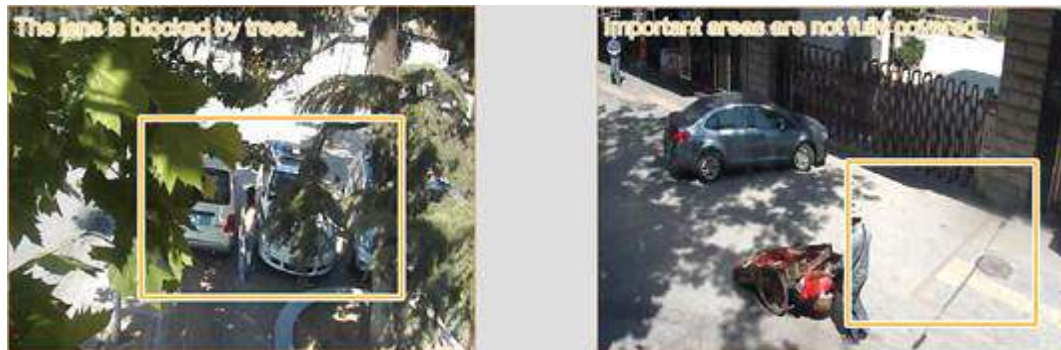
Figure 3-6 Invalid detection due to improper installation
